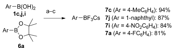
Scheme 4. Reaction conditions: a) CsF (10 M aq.; 4 equiv), MeCN, 21 °C, 1 min; b) 5 (2.05 equiv, THF) 1–5 min; c) dilute with MeCN, filter, evaporate. For 6a , MeCN/MeOH (9:1) employed.
